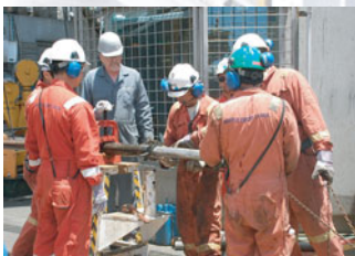
Taking out core from core barrel
