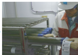
Core cut into sections
