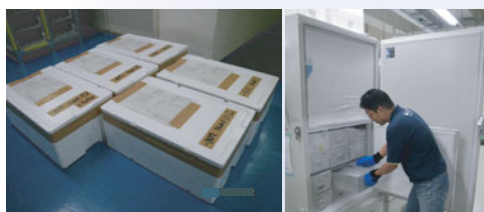
Frozen core samples transferred to KCC and stored in deep freezer (-80 °C)
