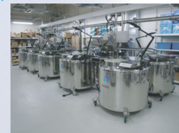
Liquid nitrogen-cooled tanks (-160 °C)
