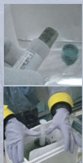
Subsampling with tip-cut syringe
