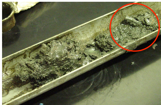
Fig.2. Ruptured plastic bag (in red circle) in a recovered core
