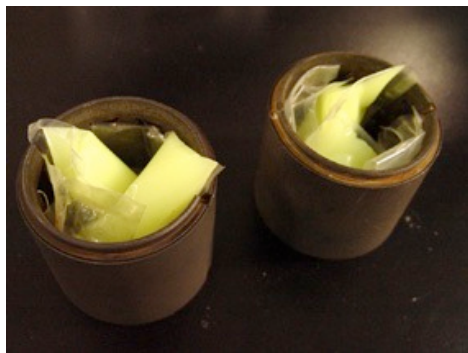
Fig.1. Plastic bags containing suspension of fluorescent microspheres, attached in core catcher
